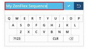
14. Select the Return Arrow in the top right corner to save the sequence and return to the main screen
