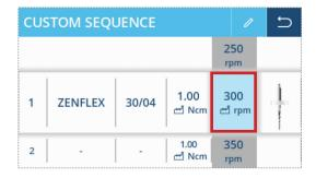
10. Select the File section of the row and the scroll to set the corresponding Tip Size band color
